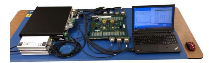
A PC running commercial ATE software, along with a DUT validation board, cables, power supplies, and two EV100 ATE-class instruments fits nicely on a lab bench.
